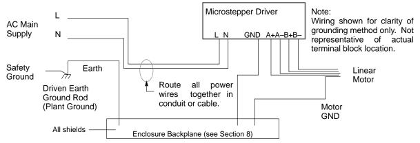
Note: Use shielded cable for driver signal wires. Route driver signal wires in conduit. These wires must be kept separate from power and motor wires.
